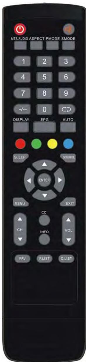
**POWER:** Power on/off button, press once to turn the TV on and press again to turn the TV off.
